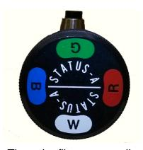
The color filters are easily selected by rotating the head of the probe.
